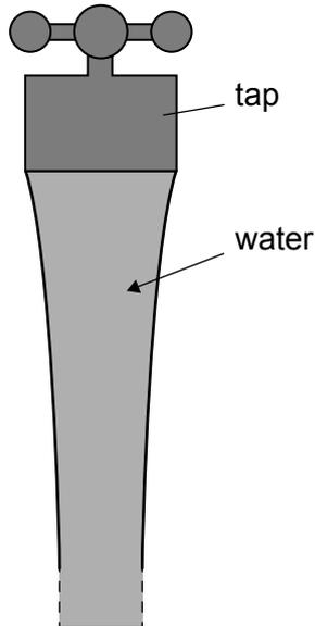
(a) Water leaves the tap at an initial speed of  $1.2 \text{ ms}^{-1}$ . Calculate the speed of the water when it has fallen 0.20 m.
